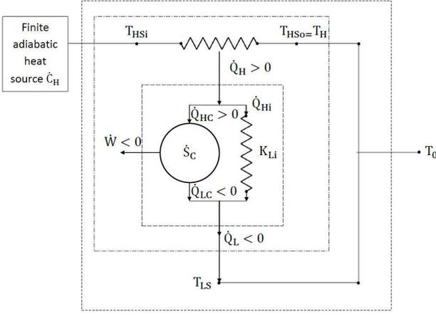
Figure 1. Chambadal power plant model
